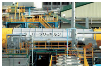
Vinyl chloride de-Cl process
