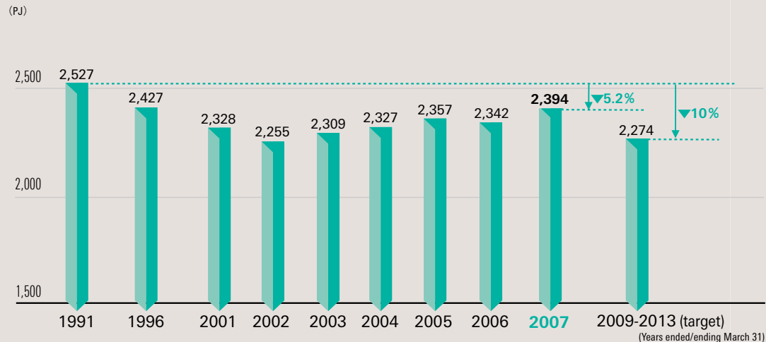
Transition in Energy Consumption by the Iron and Steel Industry in Japan
