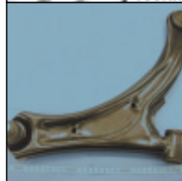
Automobile suspension components manufactured using NANO HITEN
