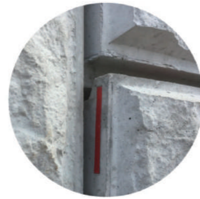
Fail-Sensor indicator (red indicating internal anomalies)
