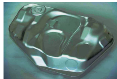
Test-manufactured fuel tank using stainless steel
