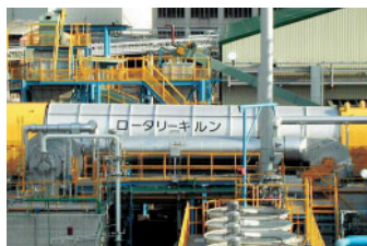
Vinyl chloride de-Cl process
