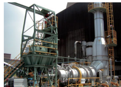
Rocking-type carbonizing kiln
