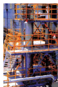
CFB test device (biomass treatment capacity: 150 kg/hr)
