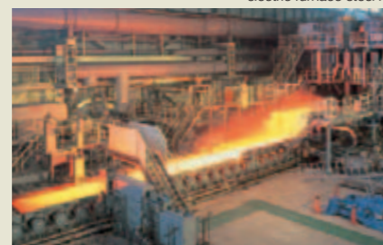
Hot endless rolling
