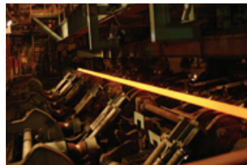
Small diameter seamless steel pipes production facility at Chita
