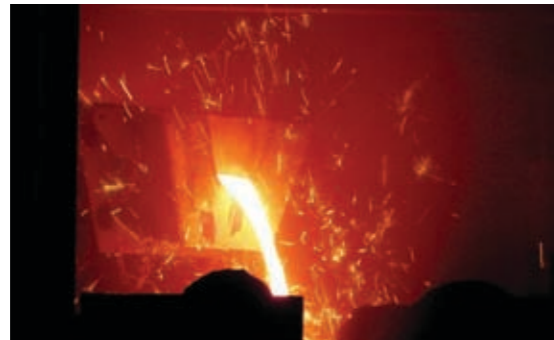
Tapping of shaft furnace in Keihin area
