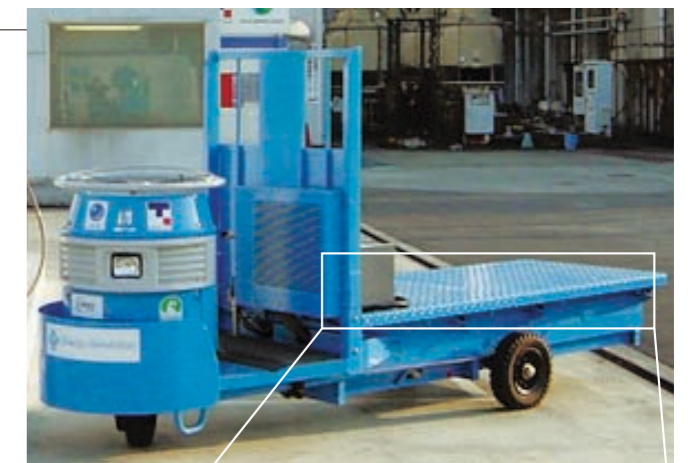
Turret cart equipped with hydrogen gas tanks
