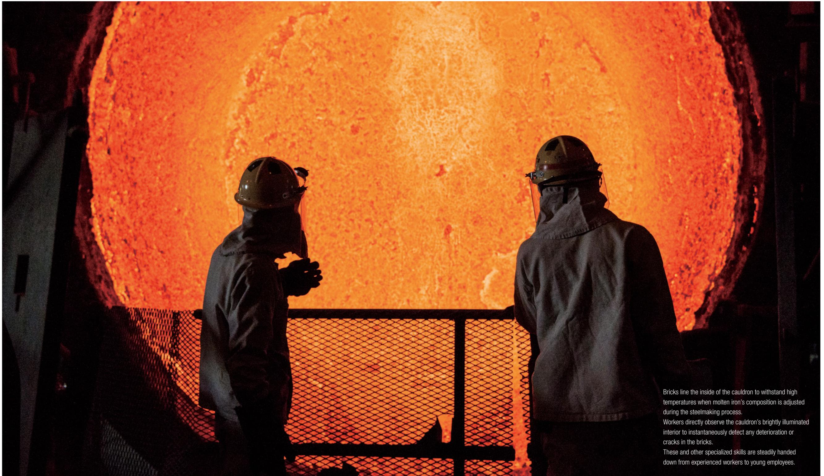
Bricks line the inside of the cauldron to withstand high temperatures when molten iron's composition is adjusted during the steelmaking process. Workers directly observe the cauldron's brightly illuminated interior to instantaneously detect any deterioration or cracks in the bricks. These and other specialized skills are steadily handed down from experienced workers to young employees.
