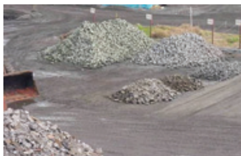
Sorted waste bricks for recycling at East Japan Works (Keihin)
