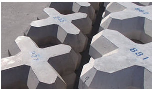
Wave-dissipating and foot protection block
