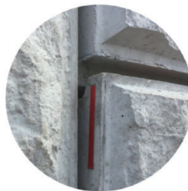
Fail-Sensor indicator (red indicating internal anomalies)
