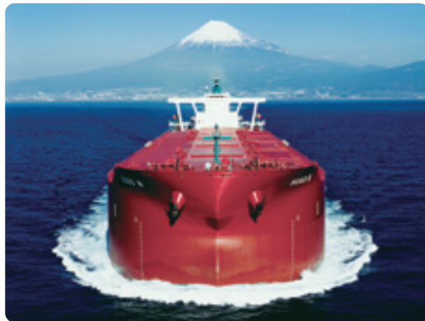
Super-sized ore carrier (specialty vessel) incorporating high-strength steel plates
