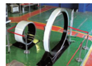
JFE product adopted for study (example) High-strength steel tubes (P-500 and P-630) for Tokyo Sky Tree® tower
