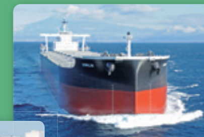
Bulk carrier equipped with LEADGE-Bow design for improved fuel efficiency (Universal Shipbuilding, page 48)
