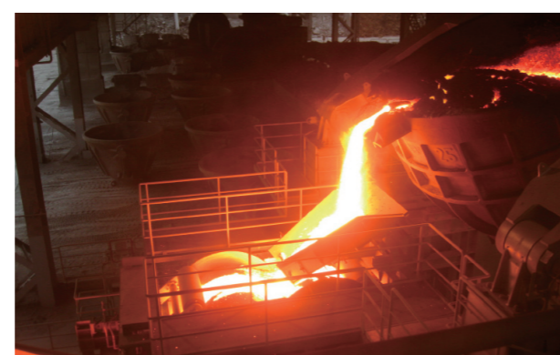
Experimental equipment for recovering waste heat from steelmaking slag (Chiba Works)
