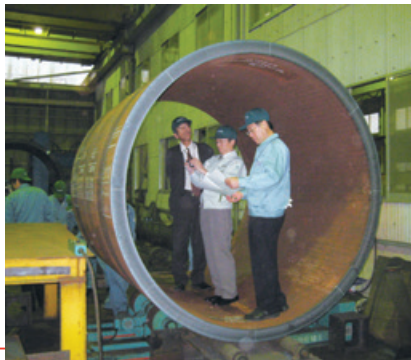
Large-diameter extra-thick round steel pipe used in the bottom part of TOKYO SKYTREE.
