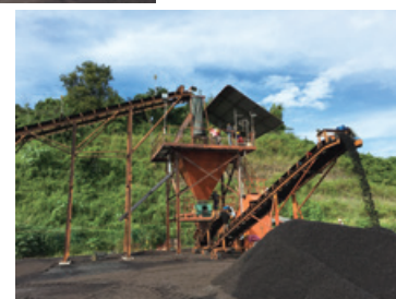
Sifter and magnetic separator to remove foreign objects
