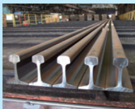
S SP3 highly wear-resistant pearlitic steel rail for heavy haul railways
