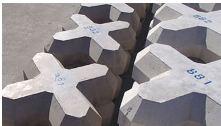
Breakwater armor block
