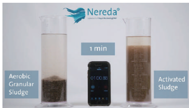
Sedimentation separation status after one minute (left: aerobic granular sludge, right: activated sludge). Microorganism-containing sludge at the bottom, purified water at the top.
