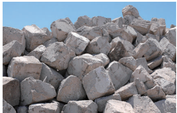
Artificial stones made from steel slag hydrated matrix
