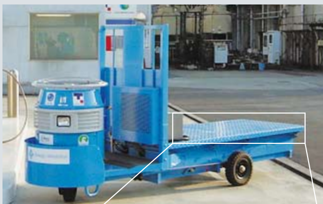
Turret cart equipped with hydrogen gas tanks
