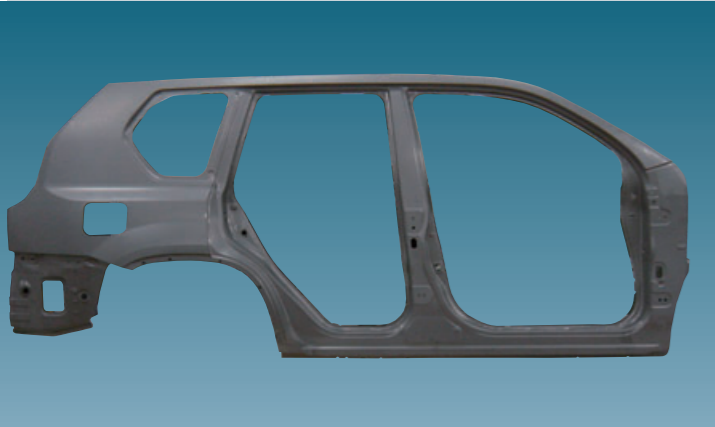
Side panel made with JAZ steel sheet
