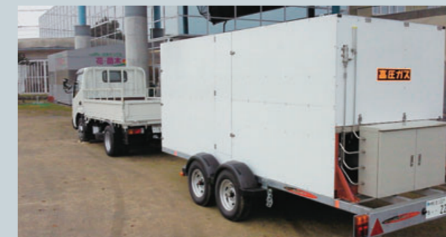
Lightweight trailer capable of transporting large volumes of biogas
