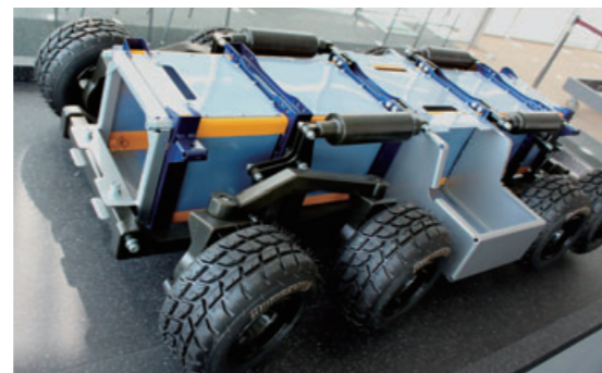
Automobile frame with built-in components for extremely compact electric vehicle
