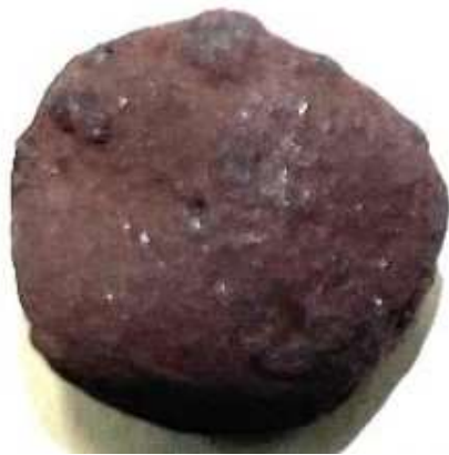
Raw material pellets Reduction rate 0% Brown
