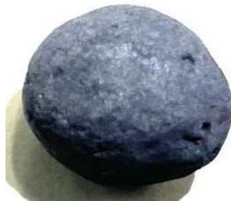
Reduced pellets Reduction rate > 90% Gray, metallic luster
