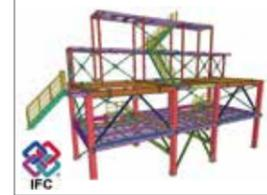
Electronic tags are attached to shipped items, and the electronic tag information is linked to 3D design data. The records of parts arrival management and construction progress are automatically obtained and used to track progress.
