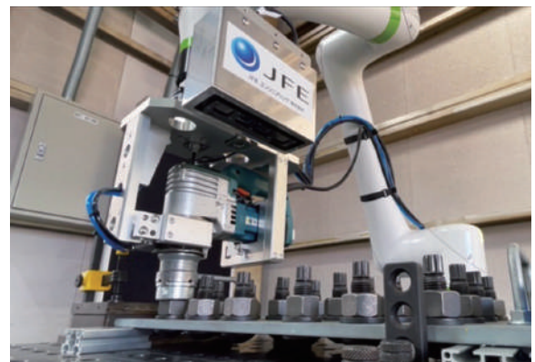
Pilot test of bolt tightening using collaborating robots
