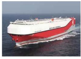
extra-wide berth suited to the expanded Panama Canal, enabling a substantial increase in cars carried by one ship. Furthermore, fuel-saving technologies reduce CO2 emissions per vehicle by approximately 25% compared to existing ships. The deck structure accommodates not only passenger vehicles, but also heavy-duty and construction machinery, railway cars and more. It now serves as the flagship of "K" Line's Drive Green Project promoting enhanced environmental performance in shipping.
