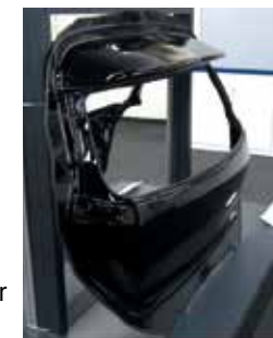
Automotive rear hatch machined with JFE Steel's new molding technique
