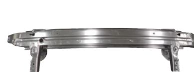
Bumper reinforcement made of 1,470 MPa-grade ultra-high-strength steel sheet
