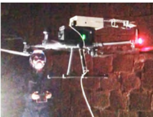
Radar-equipped drones (compatible with 1GHz~1,000GHz frequencies and bands) enable remote inspections of inside objects by exposing its properties
