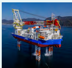
Jack-Up Vessel built by Japan Marine United
