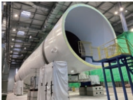
Monopile (prototype) Approx. 10-m diameter, 60-m length, and 1,000-t weight
