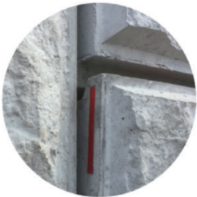
Fail-Sensor indicator (red indicating internal anomalies)
