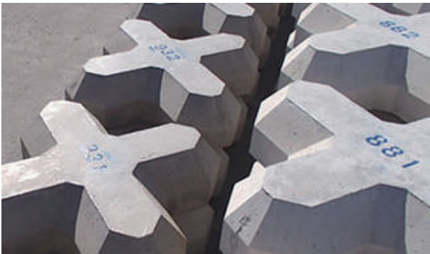
Wave-dissipating and foot protection block
