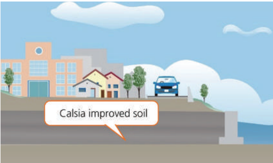
Example of calcia improvement soil application (landfill material)
