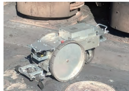
Figure 1. GAZMASTAR™ autonomous cleaning robot for harsh operating conditions
