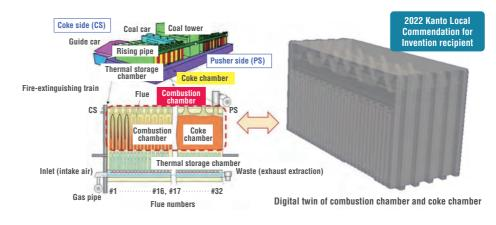
Figure 1. Digital twin model of coke furnace and its architecture
