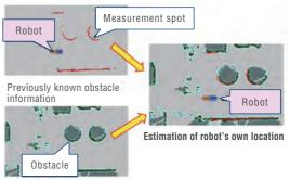
Figure 2. Use of SLAM for robot to determine its own position
