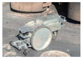
Figure 1. GAZMASTAR  $\ensuremath{^{\rm TM}}$  autonomous cleaning robot for harsh operating conditions
